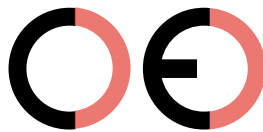
False CE Mark (too far)
